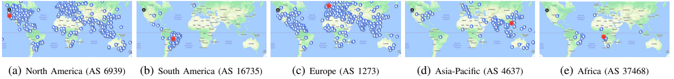
Figure 4: Maps of geographic locations of shadow ASes (blue pins) in five case studies where victim AS (black pin) is Amazon (AS 16509) and the attacker ASes (red pins) are the largest Tier-2 ASes in five continents.
